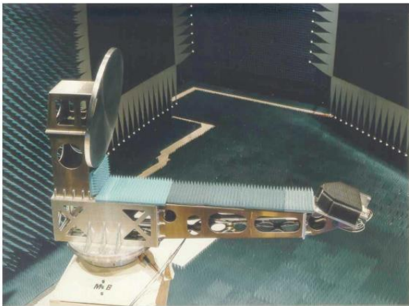
Figure 9: ADMIRALS RTO mounted on DUT Positioner of CCR 75/60. Courtesy of Airbus DS GmbH, Ottobrunn. Extracted from [5]
