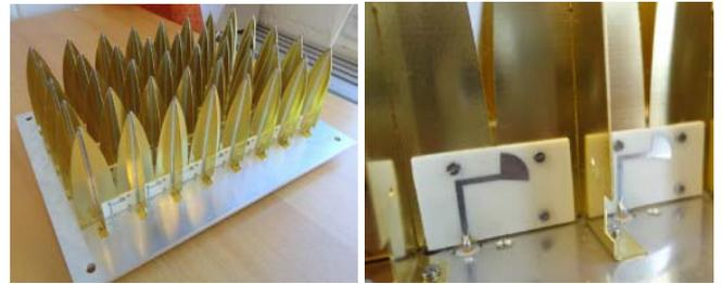
Fig. 7. Breadboard manufactured at Chalmers University, details of the feeding on the right.
