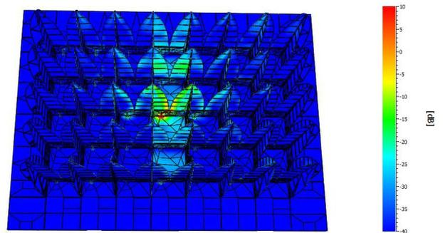
Fig. 11. Amplitude of total currents induced on the array when element 18 is excited and the other elements are matched, computed by GRASP. The dynamic range of the color scale is 50 dB.
