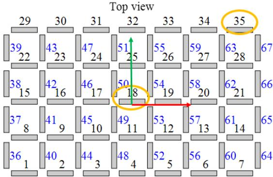
Fig. 9. Array element indexing: x-oriented Vivaldi elements are written in black and y-oriented in blue. The two elements used for pattern comparison are highlighted in yellow. The x- (red) and y-axis (green) and the origin of the reference coordinate system are shown as well.
