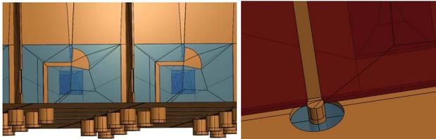
Fig. 5. Model of the breadboard in the MoM add-on to GRASP: zoom in on the microstrip and coaxial feeding.
