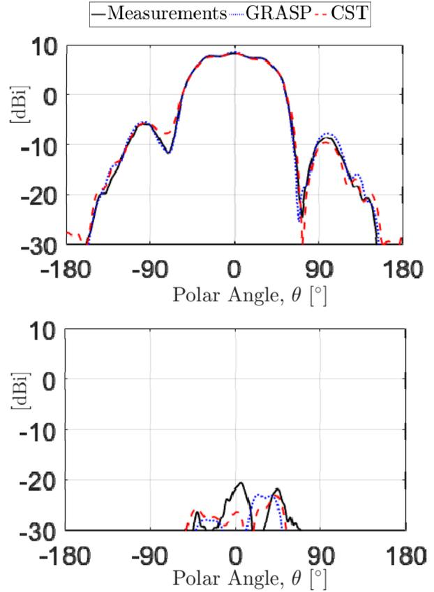
Fig. 10. Amplitude pattern in dBi in the  $\phi = 90^\circ$  cut for the center element 18 at 6.9 GHz: measured (GRASP) [CST] patterns shown in black (blue) [red]. The co-polar (cross-polar) component is shown in the top (bottom) panel.
