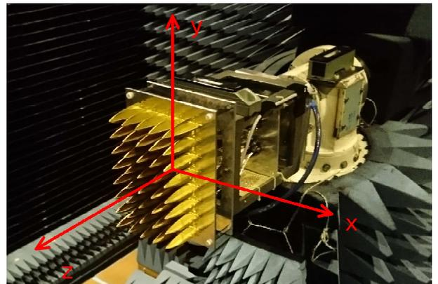
Fig. 8. Breadboard mounted on the antenna tower at the DTU-ESA Spherical Near-Field Antenna Test Facility, with the measurement coordinate system highlighted.
