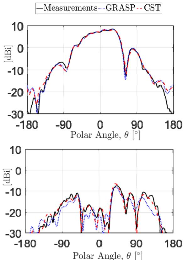
Fig. 12. Amplitude pattern in dBi in the  $\phi = 90^\circ$  cut for the corner element 35 at 6.9 GHz: measured (GRASP) [CST] patterns shown in black (blue) [red]. The co-polar (cross-polar) component is shown in the top (bottom) panel.
