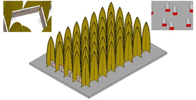
Fig. 6. Model of the breadboard in CST. All Vivaldi elements and the finite-size ground plane are visible, as well as details of the coaxial feeding.
