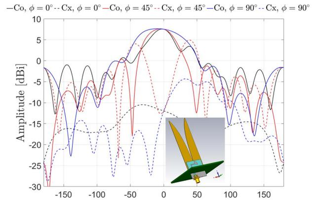
Fig. 3. Co-polar and cross-polar components of the far-field pattern of the single element computed with CST at 6.9 GHz.
