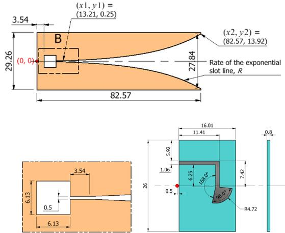
Fig. 2. Detailed geometry of the Vivaldi element: the antenna is made of aluminum with 0.4 mm thickness. The dielectric material for the PCB is Rogers RO4003 with permittivity equal to 3.55 and loss tangent equal to 0.0027. All dimensions are in millimeters (mm).
