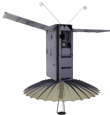
Fig. 9. The RainCube spacecraft, as available at [10].
